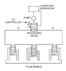
**Shunt Inlet Section.** A three-function valve, either electric or pneumatic,
