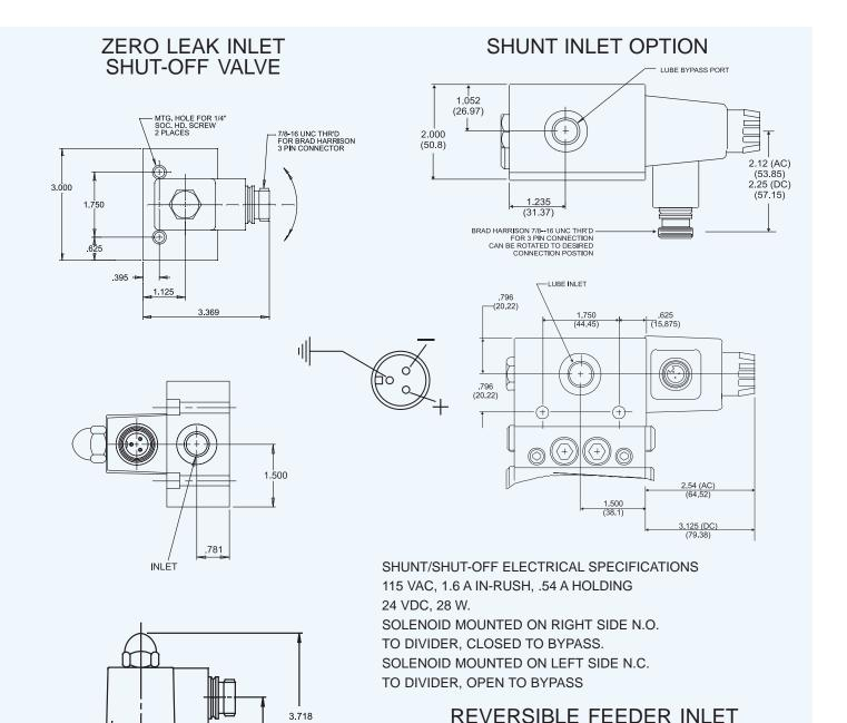
ZERO LEAK ELECTRICAL SPECIFICATIONS 115 VAC, .22 A IN-RUSH, .14 A HOLDING 24 VDC, 28 W
