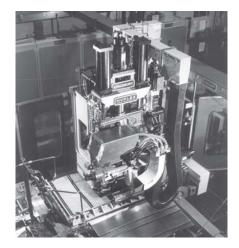
Automated systems improve safety. Maintenance personnel do not have to lubricate dangerous machinery. Operators have less exposure to oil and lubricants on equipment and floor.
